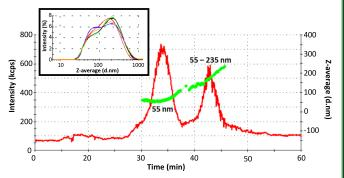
Batch-mode (inset) versus flow-mode DLS measurements of a micellar drug formulation. Multiple size populations are observed by both measurements and indicate a polydispersed sample. However, flow-mode DLS (coupled to AF4) can better measure the size distributions of each population. Adapted from Anal Bioanal Chem, 2020, 412(2), 425-428.
