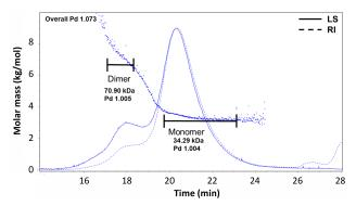
Purity assessment of drug-conjugated and targeted Generation 5 PAMAM dendrimers by size exclusion chromatography with MALS and refractive index detectors in-line (SEC-MALS-RI). The molecular mass distribution and polydispersity for the monomer and dimer are based on the bracketed molar mass distribution.
