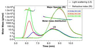
Polymer composition and molar mass distribution of mPEG-PLGA were determined by thermogravimetric analysis and SEC-MALS-RI (above), respectively.
