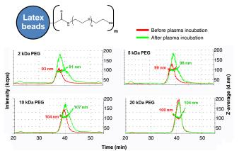
Flow-mode DLS, coupled to AF4, of polystyrene beads conjugated to various lengths of PEG before and after incubation in human plasma. As PEG length increases, polydispersity decreases and there is minimal change in the size distribution pattern (red vs green trace), suggesting decreased protein binding with increased PEG length.
