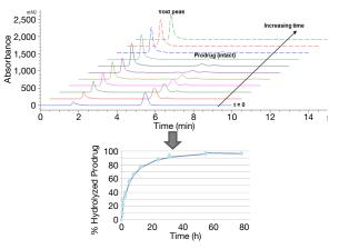
Stability assessment of prodrug micelles in the presence of human plasma. The hydrolysis of the intact prodrug was measured by RP-HPLC and used to construct a hydrolysis versus time graph, which can be used to determine  $t\frac{1}{2}$ .
