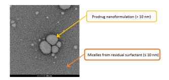
Representative TEM image of PEGylated oil-filled prodrug nanocapsules. In addition to determining the size distribution, TEM can be used to evaluate morphology and purity. Here, the presence of residual surfactant forming smaller micelles are observed in the background.
